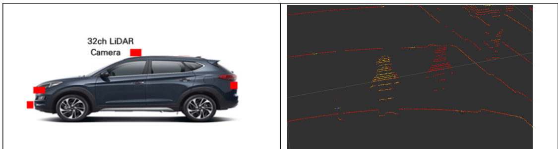
<Fig. 3> LiDAR Sensor Equipment and Human sign's PCD example
