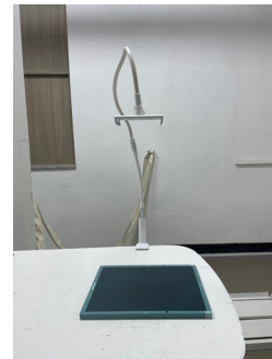
Fig. 2. Fixed holder for photography
