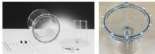
Fig. 2. Triple line insert phantom was used to evaluate the total count of SPECT/CT study
