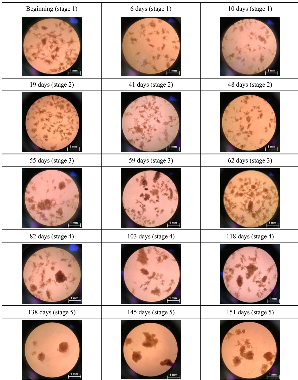
Fig. 5. Morphology observation of AGS during the operation periods in the pilot plant. 40 magnification by optical microscope.
