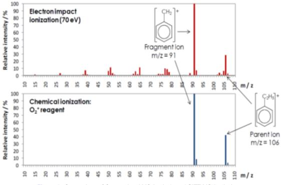
Figure 3: Comparison of Conventional MS Analysis and SIFT-MS Analysis
