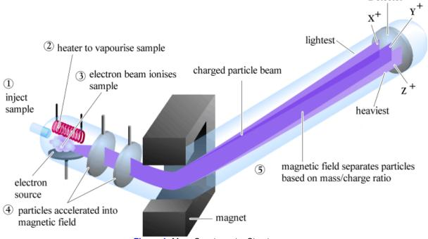
Figure 1: Mass Spectrometer Structure
