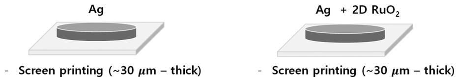
Fig. 3. Schematic diagram of the Ag current collectors coated on alumina substrate.
