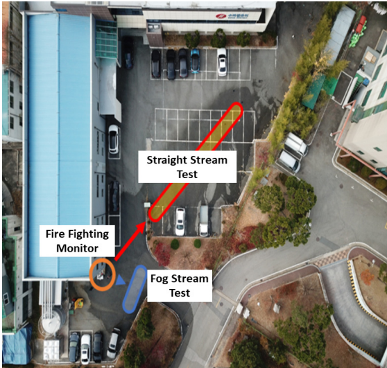
Fig. 7 Bird-view of test region for water spray test of fire fighting monitor
