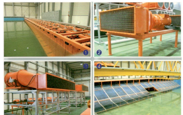
Fig. 4 Experimental equipment : ① Wave maker, ② Current generator, ③ Wind generator, ④ Wave absorber
