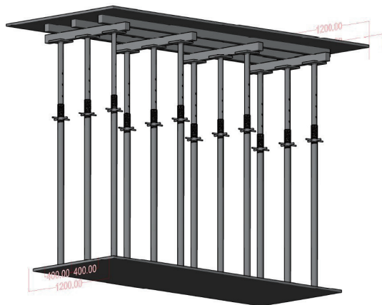
Figure 4. Three-dimensional formwork model in AutoCAD
