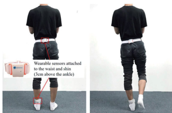
Figure 2. Marker models for the Inertia Measurement Unit sensor (IMU) for the one leg standing test.
