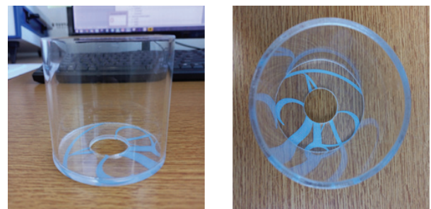
Fig. 4. Acryl mold for the mortar specimen
