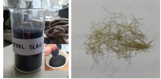
Fig. 3. Steel slag(left) and fibers(right) used
