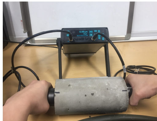
Fig. 4. Ultrasonic pulse velocity measurement
