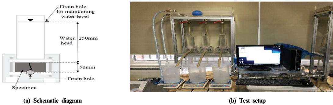
Fig. 4. Water permeability test
