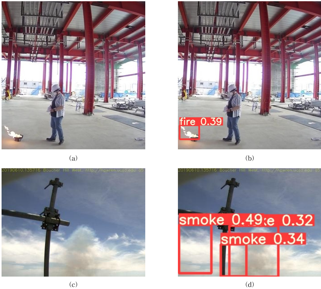
Fig. 8. Results of performing unstructured object recognition, (a), (c) A screen in which unstructured objects are not detected when performing the first object detection and (b), (d) A screen with object detection through video integration analysis.
