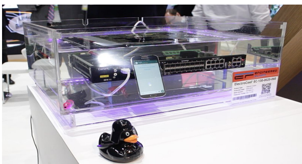
Fig. 1. Single-phase, liquid immersion cooling
