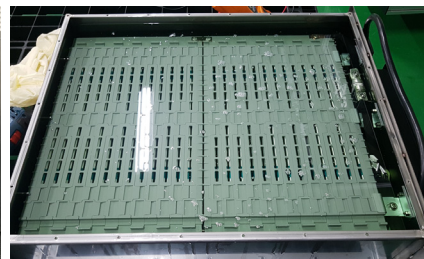
Fig. 4. Immersion cooling test specimen
