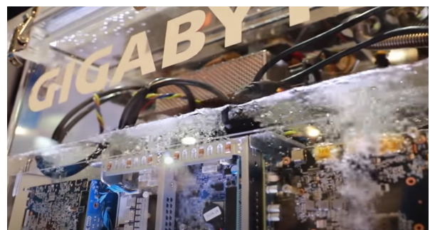
Fig. 2. Two-phase liquid immersion cooling
