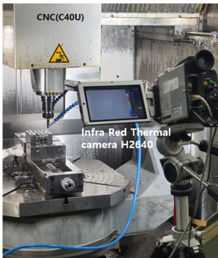
<Figure 2> Measuring Cutting Temperature on the Machine
