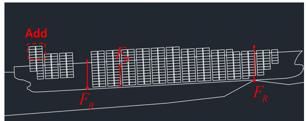
Fig. 18 New attitude of the stranded ship by cargo addition
