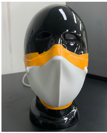
Figure 2. Photograph to measure inhalation resistance
