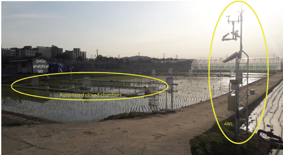
Fig. 1. A picture showing the automated closed chambers system and Automatic Weather Station (AWS) located in Gyeonggi-do Agriculture Research and Extension Services.
