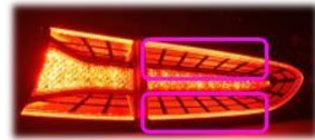
Fig. 14 lacking brightness due to insufficient light diffusion
