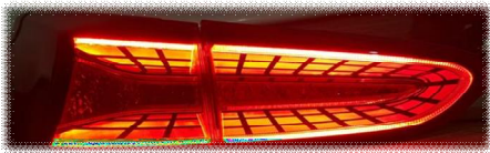
Fig. 17 New TIR lens application improvement sample
