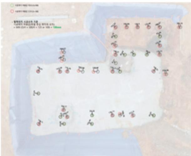
Fig. 11. Analysis Result of Pile Foundation Construction Error
