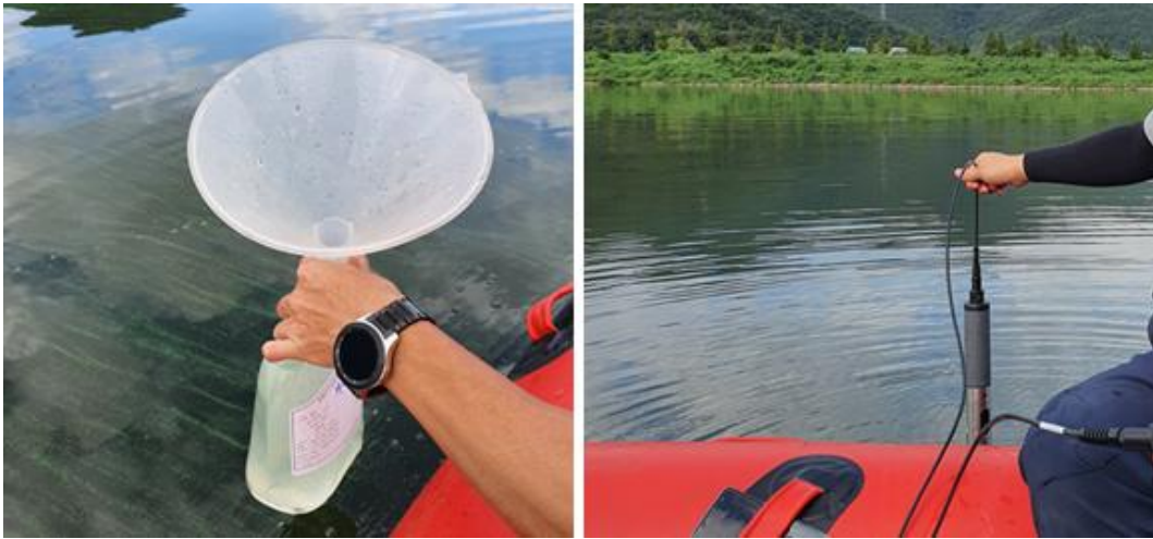
FIGURE 5. Field works: river water sampling(left) and in-situ measurements(right)
