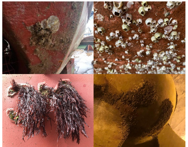
Fig. 5. Examples of biofouling cover on hull and bow thruster rim on the ship B, C, D and E. (a) Heavy macrofouling on bow thruster rim, (b) barnacle on the bottom, (c) macroalgae on the hull and (d) barnacle on the propeller.
