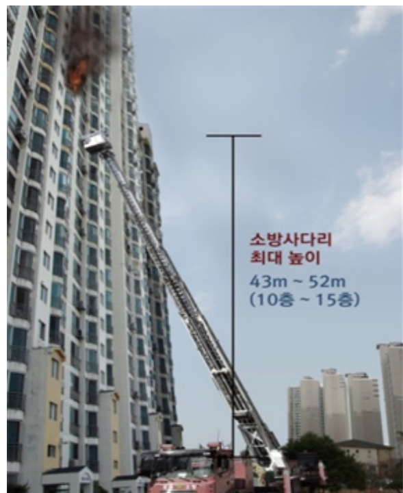
〈Fig. 3〉 Limitations of fire ladders in case of the fire
