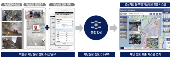
Fig. 5. A diagram of the connection between the disaster site information collection application and the disaster information display system
