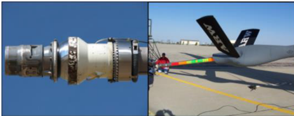
Fig. 3 Boom Nozzle & Ruddervator [5]
