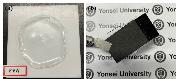
Fig. 2. Photographs of (a) PVA/H 3 PO 4 free-standing membrane and (b) assembled solid-state supercapacitor.
