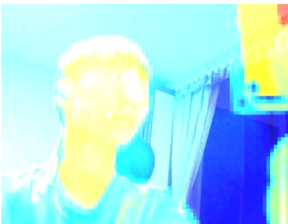
Fig. 2 The result of synthesizing the image of the thermal imaging camera and the camera after positioning and cropping
