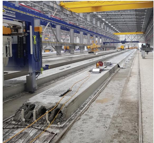
Fig. 3. Shape of HCS member before cutting
