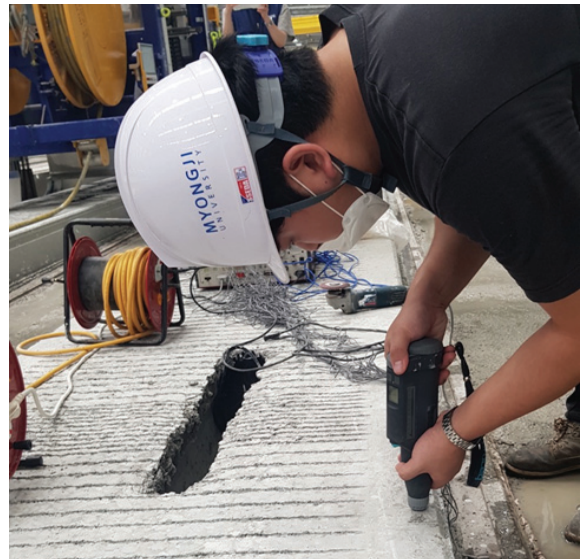
Fig. 4. Measurement of compressive strength of concrete using schmidt hammer
