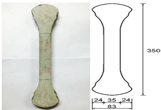
Fig. 2. Detail of specimen for direct tensile test
