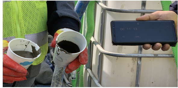
Fig. 2. Gel time of rapid hardening cement (11 sec, cup shifting method)
