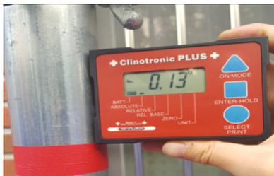
Fig. 5. Digital inclinometer(Clinotronic PLUS) and Measured slope.
