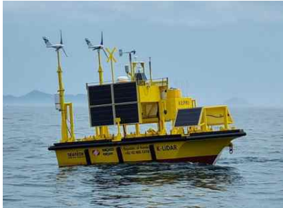
Fig. 19 Floating LiDAR buoy (Real installation picture)
