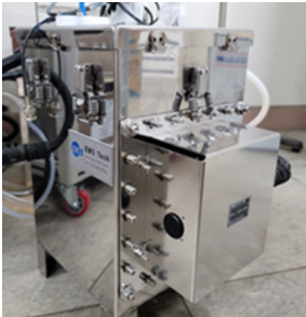
Fig. 1. Reactor coupled with a pair of ultrasound transducers
