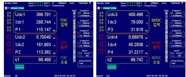
Fig. 11. Measured efficiency at full load.
