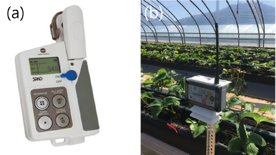
Fig. 1. Data collection device (a) Chlorophyll meter; (b) Temperature and humidity wireless sensor.
