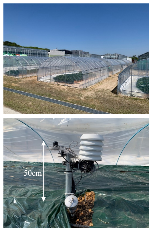
Fig. 1. The greenhouse (left) was structured by iron pipe with 1.3 m eave height and 2.5 m ridge height, and covered with 0.15 mm thick plastic film having the surface area of 40 m 2 with 5 m width and 8 m length, which was equipped with rolling type side window operated by the temperature sensor located at the center of greenhouse on 1.5 m height. Microclimate sensors (right) used for this experiment.
