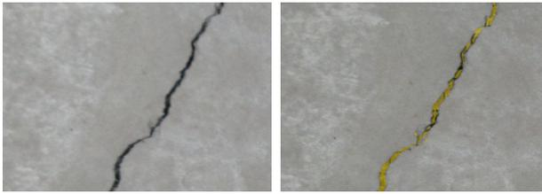
Fig 10. Comparison of Detection Result with Crack in Original Image
