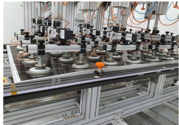
Fig. 1. Mechanical load test system in this study
