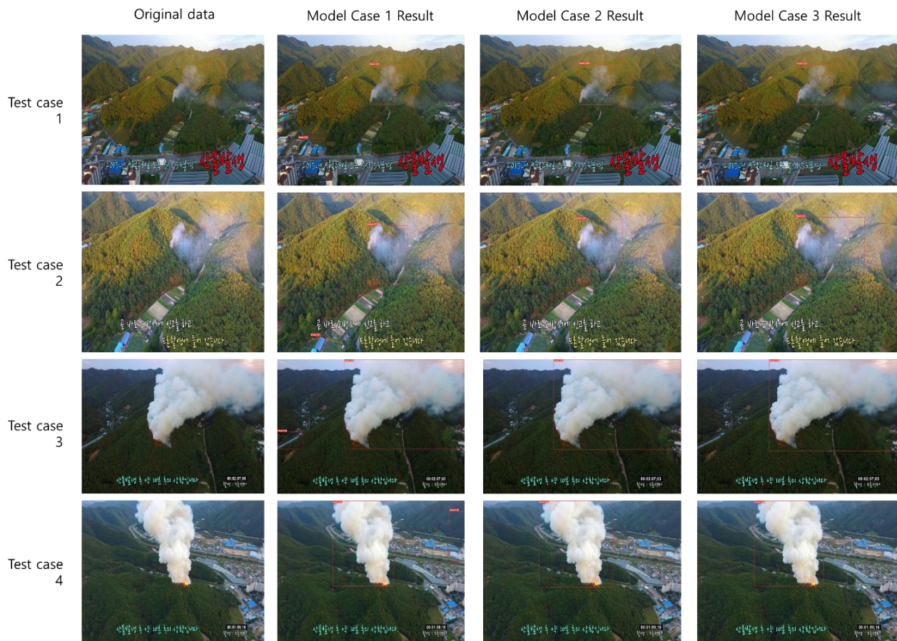
Figure 9. Actual Wildfire Smoke Detection Results for Each Model Case
