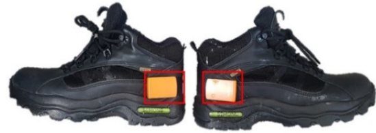
Fig. 5. Location of the inertial sensors.
