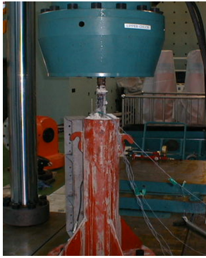
Fig. 2. Tendon-grout bond failure
