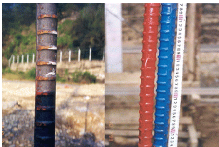
Fig. 8. Rod tensile failure (Moderately weathered, depth=6.0m)
