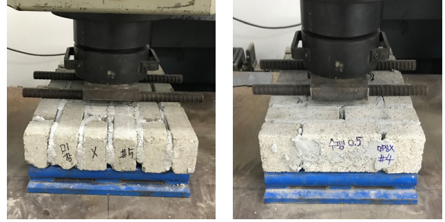
Fig. 7. Flexural tensile strength test on masonry prism, (a) failure normal to bed joint, (b) failure parallel to bed joint
