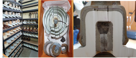
Fig. 1. Excerpt from the insulator, the insulator cut with a water jet, and the cross section of the insulator.
