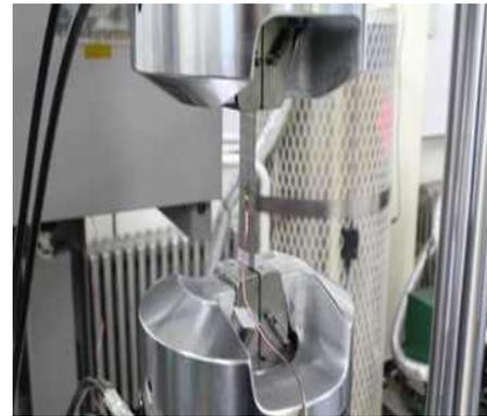
**Fig. 6** Tensile Experiment of TWF Composite
