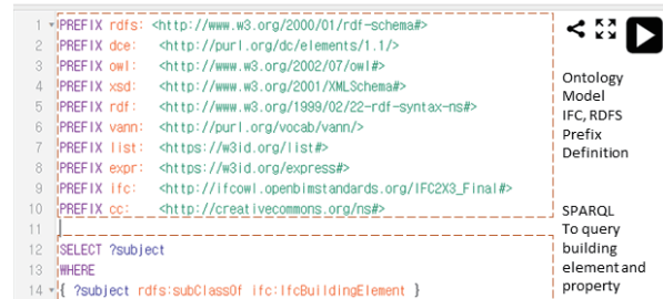
Figure 9. Ontology BIM-based BIM information query example
