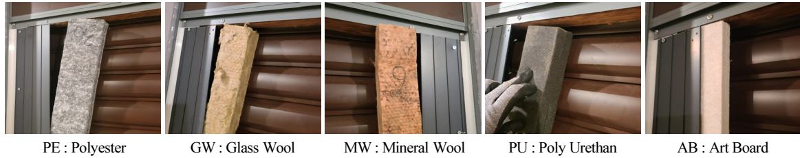
Fig. 7. (Color available online) Sound absorbing material construction and measurement.
