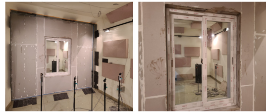
Fig. 4. (Color available online) Normal window sound insulation performance measurement.
