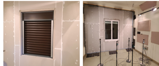
Fig. 5. (Color available online) EEB Sound insulation performance measurement.
