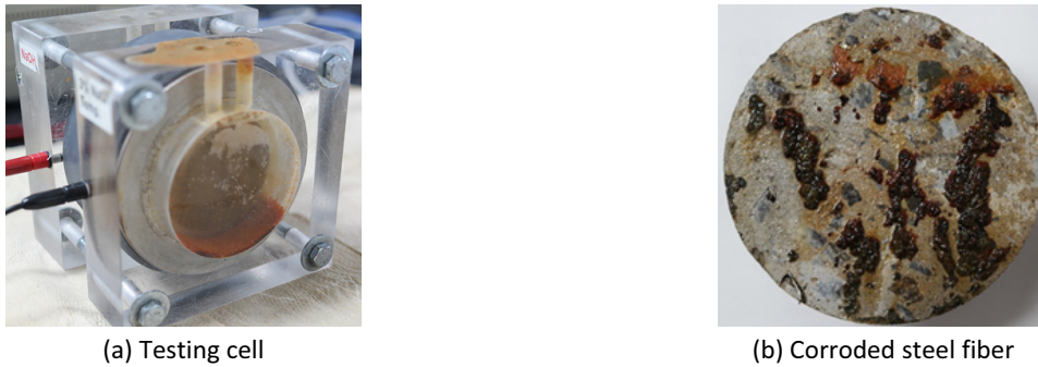
Figure 4. Photographic images obtained from ASTM C 1202 test of steel fiber reinforced concrete
