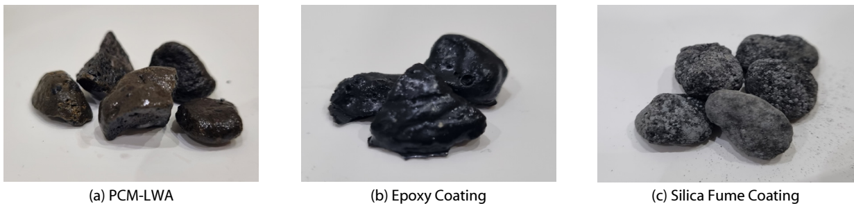
Fig. 1. Physical Appearance of the Phase-Change Material Lightweight Aggregate (PCM-LWA) As It Undergoes Two Coating Stages
