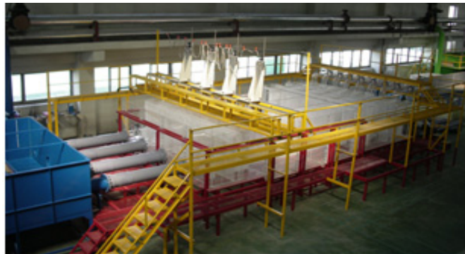
Fig. 2. Hydraulic Model of Circulating Water Intake Basin
